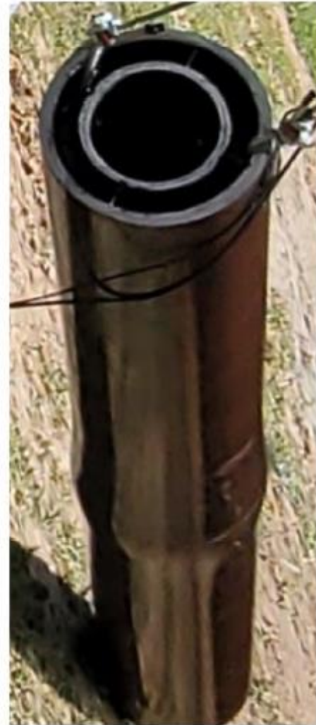
7 5/8" O.D. x 6.625" I.D., 39#, Q-125 11 3/4" O.D. x 10.282" I.D., 82.69# Q-125
